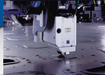
6,000 watt fiber optic laser with automation plus 2 4,000 watt lasers with 9-shelf tower system to manufacture lower to medium volume requirements.
